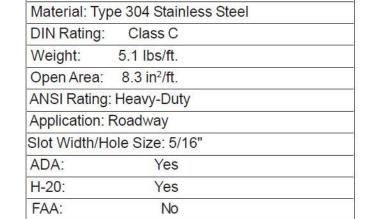
RPSRC - Reinforced Perforated Reverse Punch
